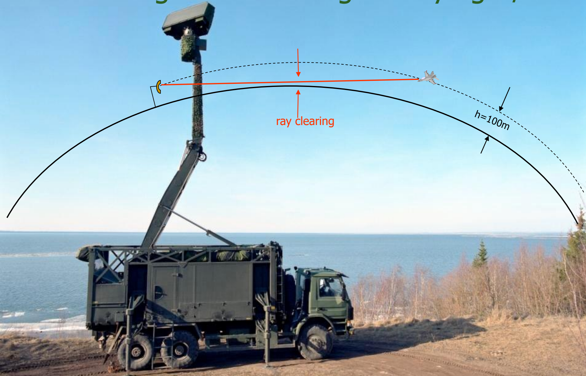
Giraffe, surveillance radar
