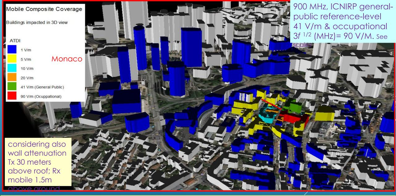
Environmental levels: 3D cellular contours, showing buildings impacted; preliminary draft new Report ITU-R SM.[EMF-MON] 'EMF measurements to assess human exposure' Fig. 6
