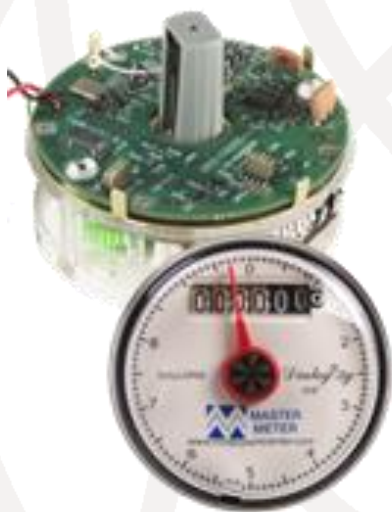
Water meter with built-in AMR radio module
