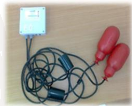
Wireless wastewater & sewage level monitoring unit with tilt sensors
