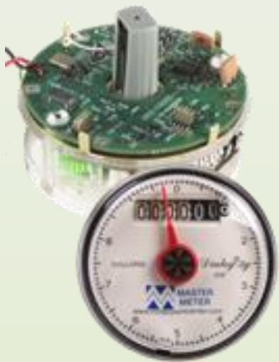
Water meter with built-in AMR radio module
