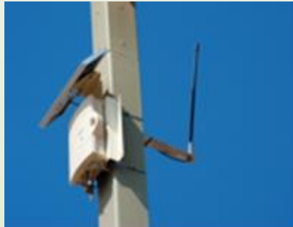
Solar-powered wireless relay for AMR
