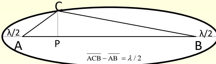
$$\overline{ACB} - \overline{AB} = \frac{\lambda}{2} \quad \overline{AC} = \sqrt{(d_1)^2 + (F_1)^2} \quad \overline{CB} = \sqrt{(d_2)^2 + (F_1)^2} \quad \text{therefore}$$
