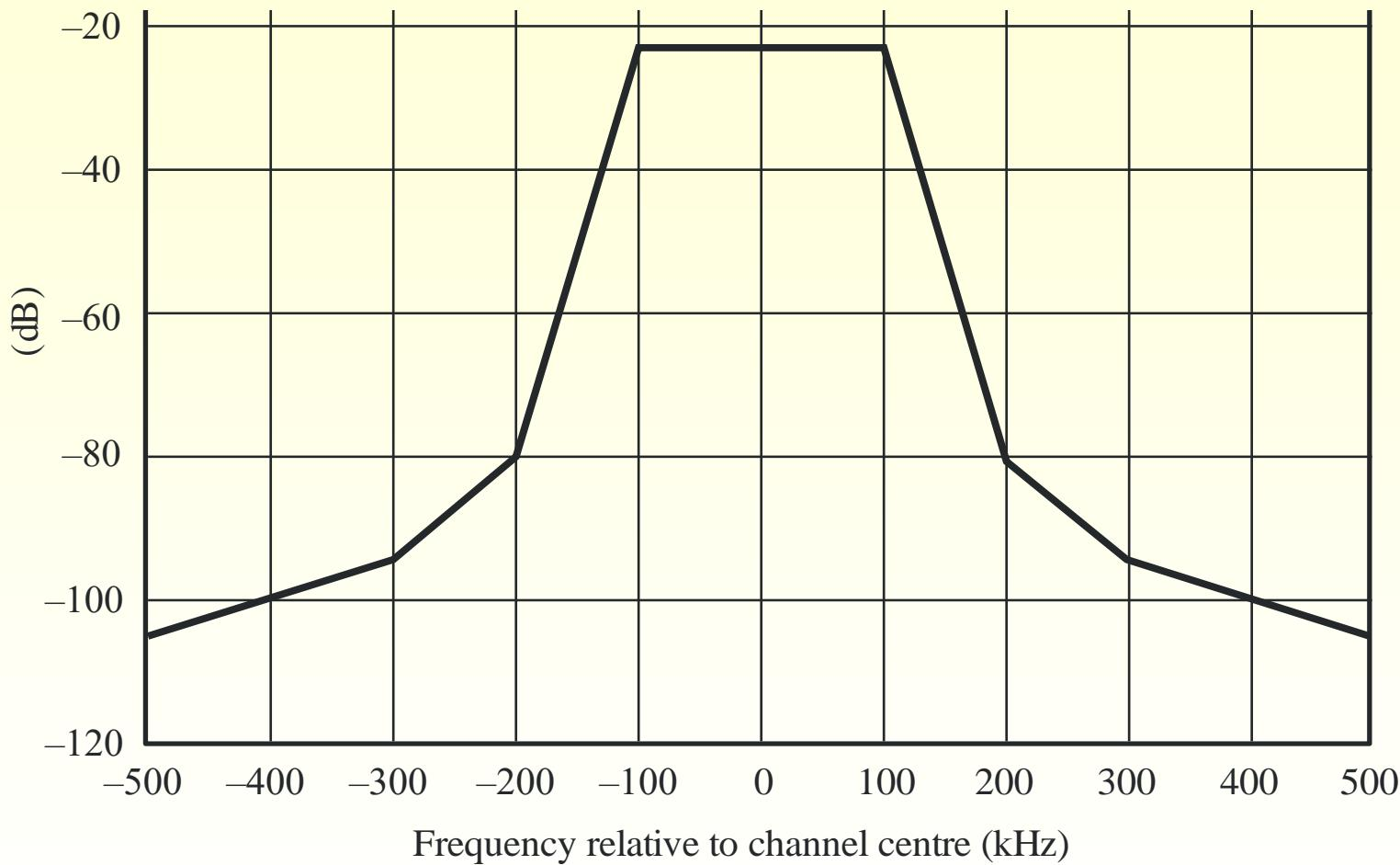
Limit mask for VHF FM sound broadcasting transmitters, 200 kHz channeling
