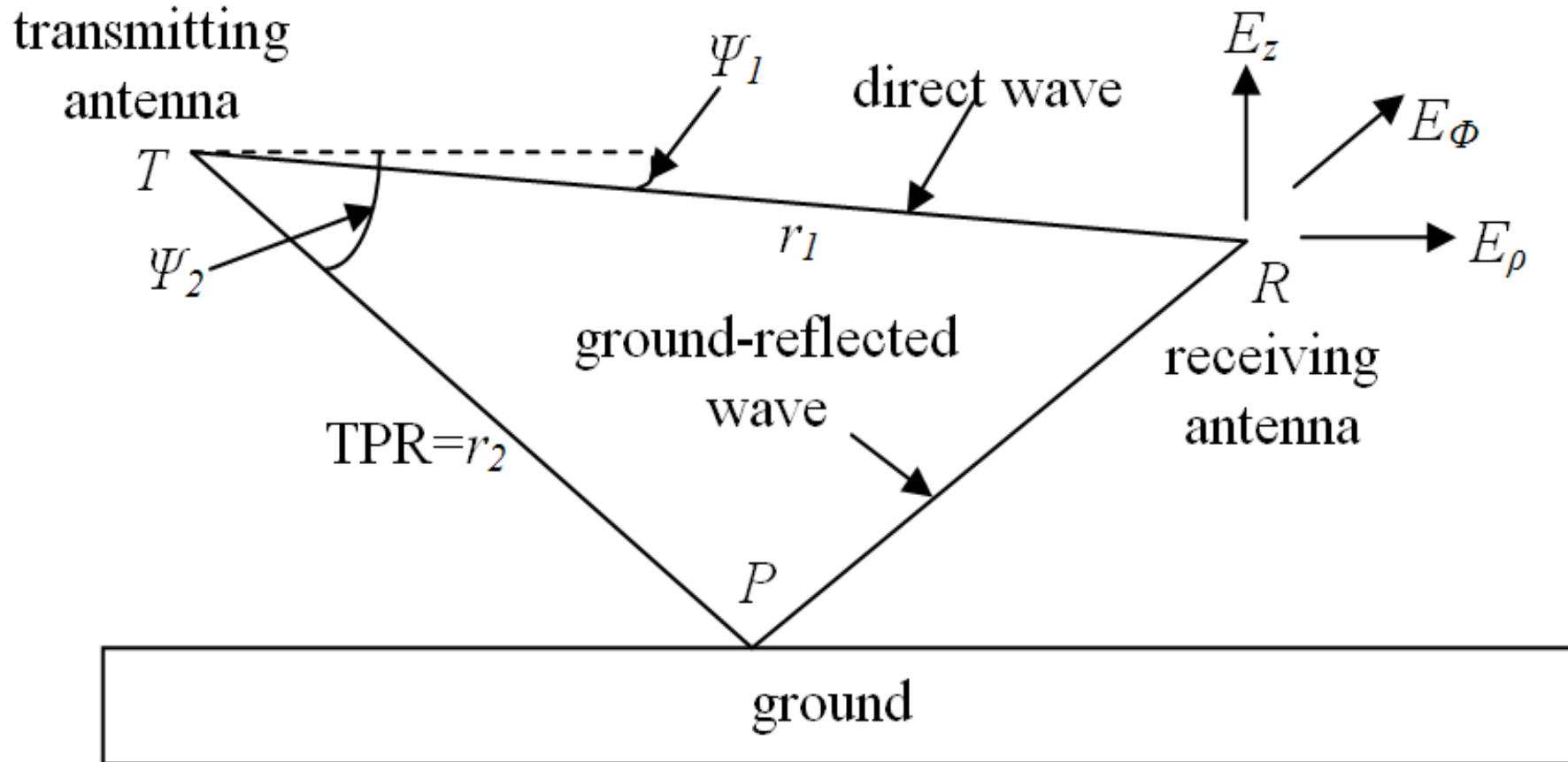
GRWAVE generates propagation curves; calculation of ground-wave field strength in an exponential atmosphere as a function of frequency, antenna heights and ground constants; approximate frequency range 10 kHz-10 GHz. GRWAVE is most useful for RF 10 kHz to 30 MHz
