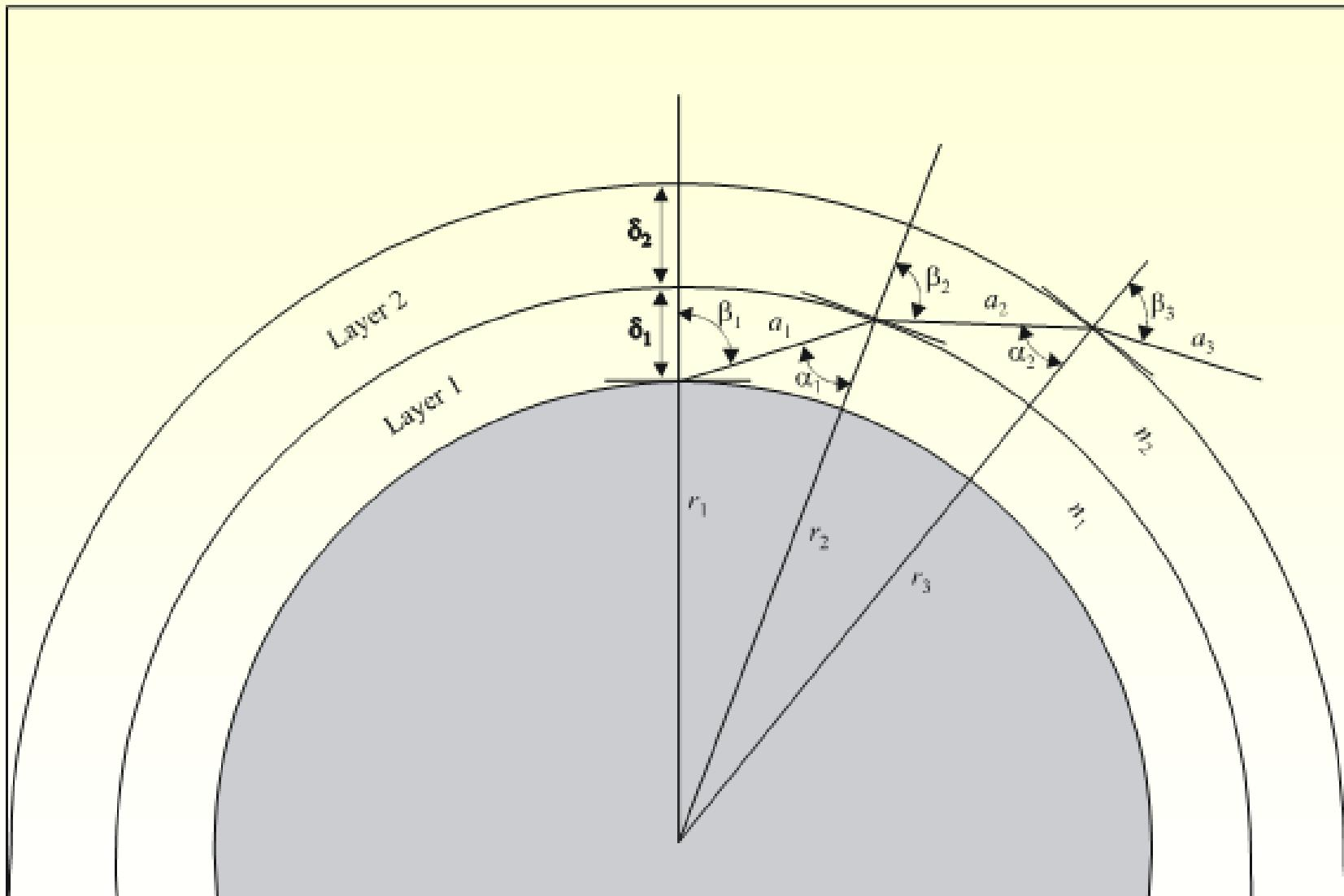
Bending of the signal (ITU-R P. 676 Fig. 4)
