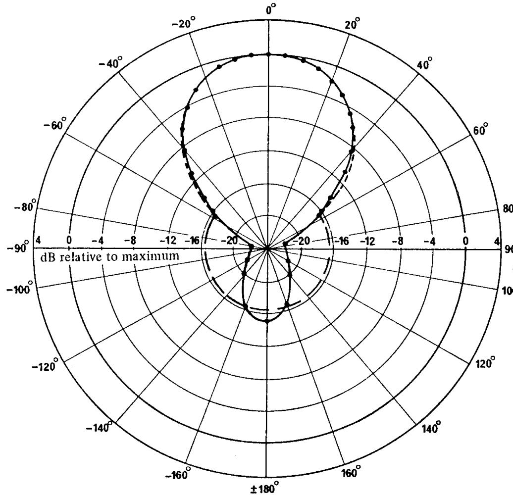
a) Azimuthal pattern HR 2/4/0.5, maximum gain 19 dBi
