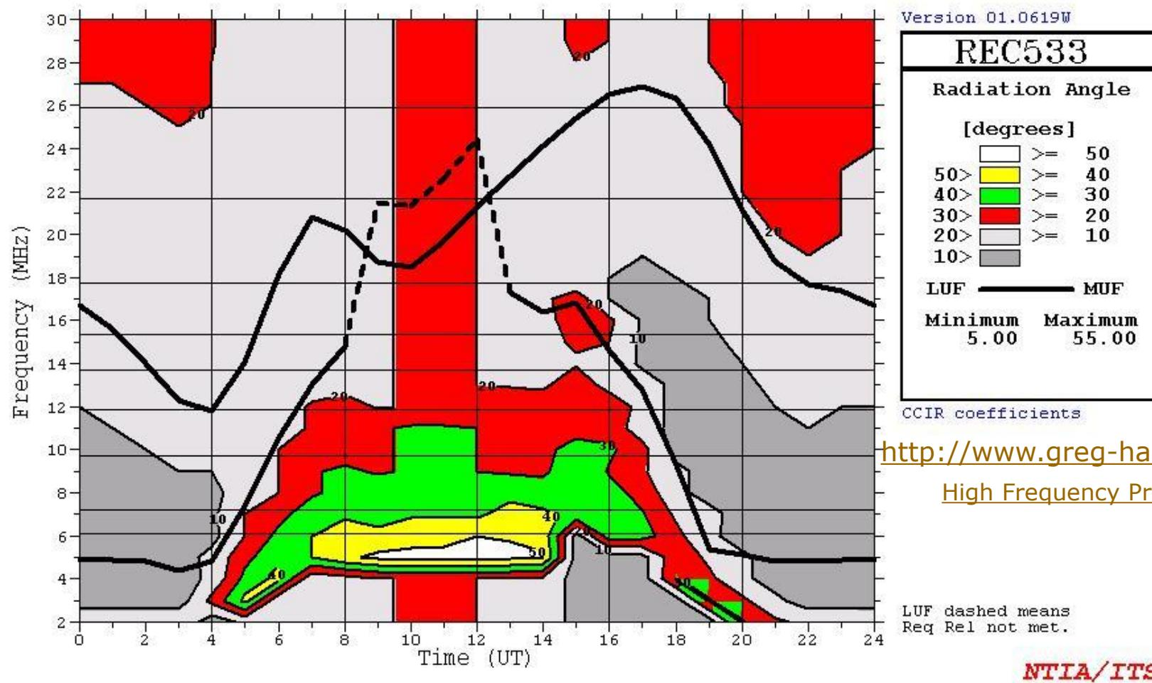
Calculated field strength (within 24 hours) in the measuring point in Moscow region Kaliningrad; Tx (NTIA@
