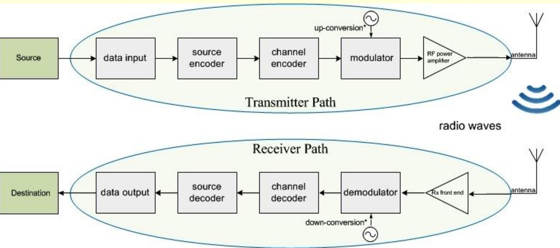
The modulation, and the up-conversion and down-conversion are not always merged; there are many structures where a signal, that is already modulated, is up-converted in a separate (mixer-based) stage.
