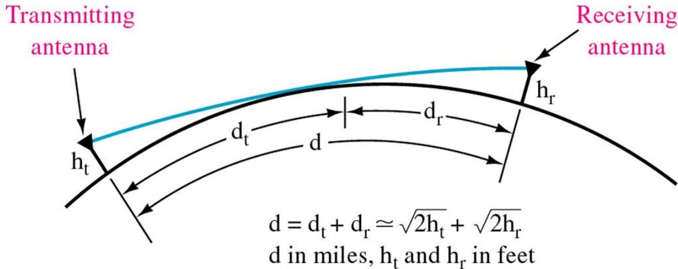
$$(a+h_1)^2 = a^2 + 2h_1a + h_1^2 = x^2 + a^2 ; 2h_1a + h_1^2 = x^2$$
