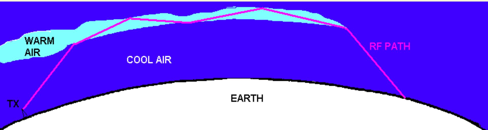
1. **Certain weather conditions** produce a layer of air in the Troposphere that will be at a higher temperature than the layers of air above & below it.
