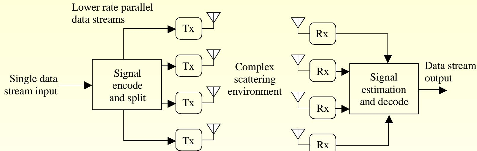
MIMO increases system throughput data rate for the same total radiated power & channel bandwidth 2038-01
