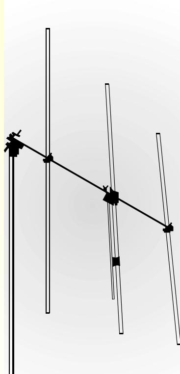
a) Typical Yagi antenna for full Band II coverage
