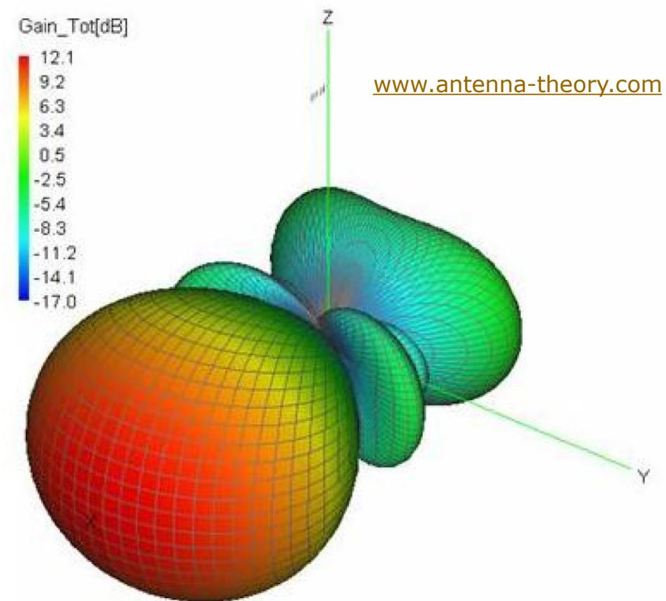
**Antenna** is the interface between **electro-magnetic waves** propagating through space and electric currents moving in metal conductors, used with a **transmitter** or **receiver**
