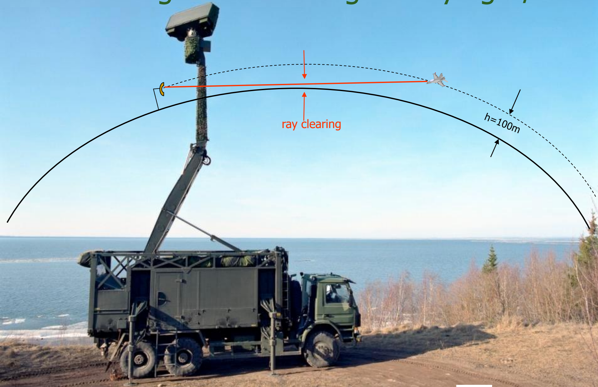
Giraffe, surveillance radar
