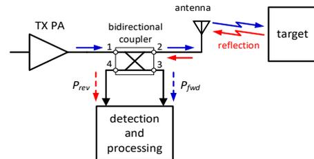
Fig. 5. Target detection system based on a bidirectional coupler providing samples of incident and reflected TX power.
