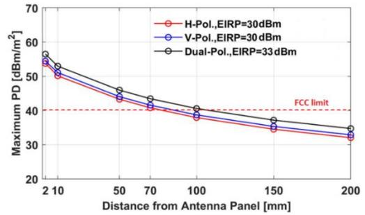
Fig. 3. Estimated power density (PD) versus distance for a device operating in FR2 capable of reaching  $\text{EIRP}=30 \text{ dBm}$  in both horizontal and vertical polarizations, adding up to a total of  $33 \text{ dBm}$ .
