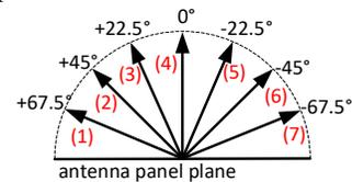
Fig. 4. Example of beamforming capability in a handset, showing 7 different possible directions for transmission in one plane (one-dimensional phased array shown with  $22.5^\circ$  steps).
