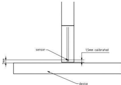
Fig. 2. Sensor of near-field probe measures the electric field within 2 mm distance from the boundary of the device-under-test (DUT).
