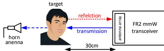
Fig. 6. Experimental setup with human head placed in boresight of a handset's mmW module, obstructing its reception in a horn antenna.
