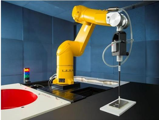
Fig. 1. Power density (PD) measurement setup based on robotic arm holding near-field EM probe (EUmmWV2, offered by SPEAG) for measurement of a device's emissions (from speag.swiss website).
