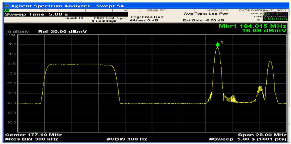
CATV QAM 256, white noise (below and above the QAM) & analog TV
