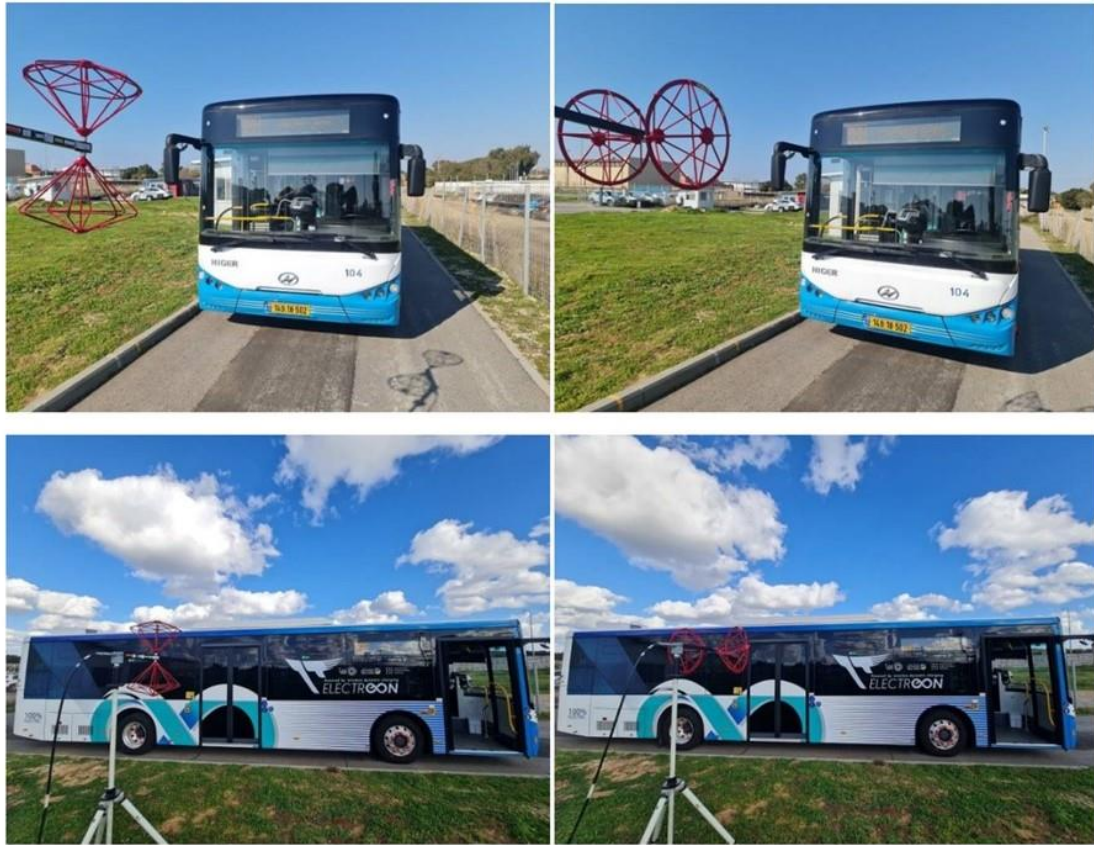
Figure 1-2 The set up for radiated emission measurements, 30 – 1 000 MHz , front and right sides
