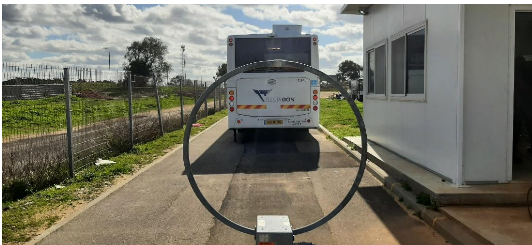
Figure 1-1 The Higher bus in Neurim, 9 kHz – 30 MHz measurement loop antenna, rear side
