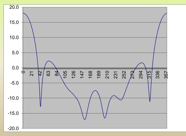
Field Strength (dBµV/m) vs. distance (m), co-located site TV, IMT 850 & Point 2 Point
