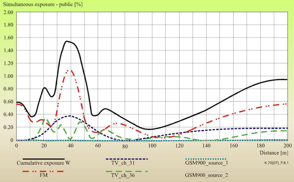
black solid line: cumulative exposure ratio  $W_t$  calculated by author; see where is max exposure 19 dotted coloured lines: contribution from each transmission component
