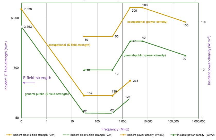
Note: the unit of the figure's left-side is electric field-strength V/m, & the right-side is W/m<sup>2</sup> power-density
